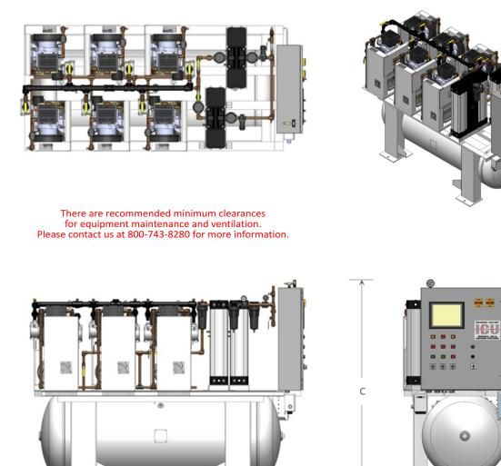
SHOWN: Duplex 15 HP, 240 gallon, horizontal tank mount, Scroll configuration with PLC shown.
