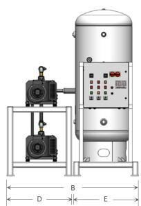
SHOWN: Duplex 6.4 HP, 200 gallon, vertical stack mount, standard dry rotary claw configuration.
