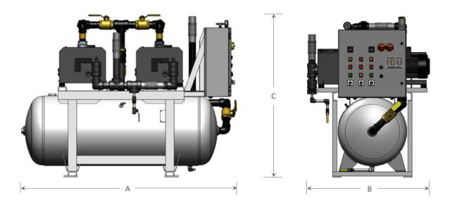
SHOWN: Duplex 6.4 HP, 120 gallon, horizontal tank mount, standard dry rotary claw configuration.
