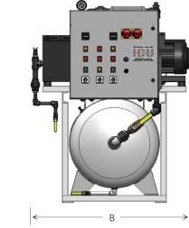
**SHOWN:** Duplex 5.4 HP, 120 gallon, horizontal tank mount, standard dry rotary claw configuration.
