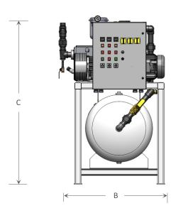
SHOWN: Triplex 10 HP (H.D.), 240 gallon, horizontal tank mount, standard lubricated rotary vane configuration.
